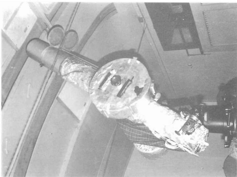
Fig. 24. The Zenith telescope "Ascania" 110/1287 mm.
