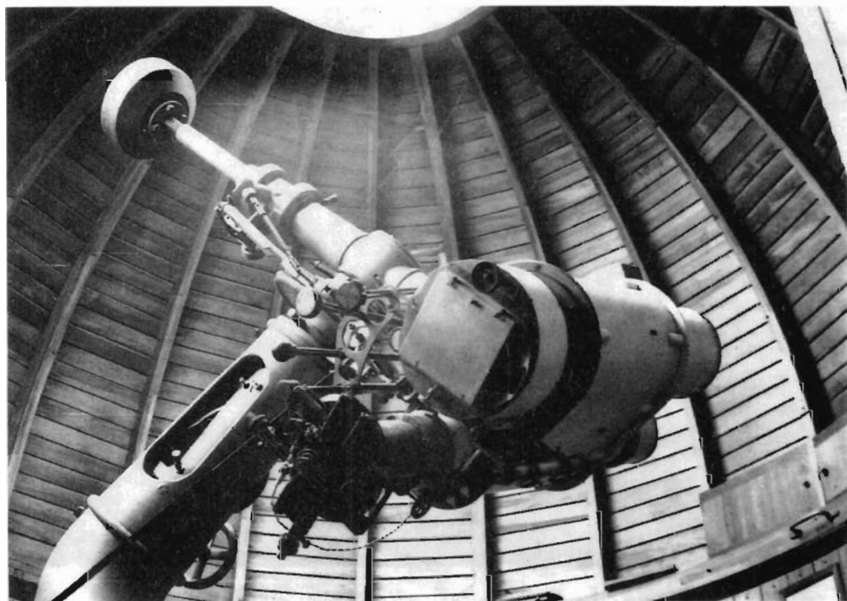
Fig. 10. Photovisual refractor "Ascania" 135/1000 and 125/1000 mm.
