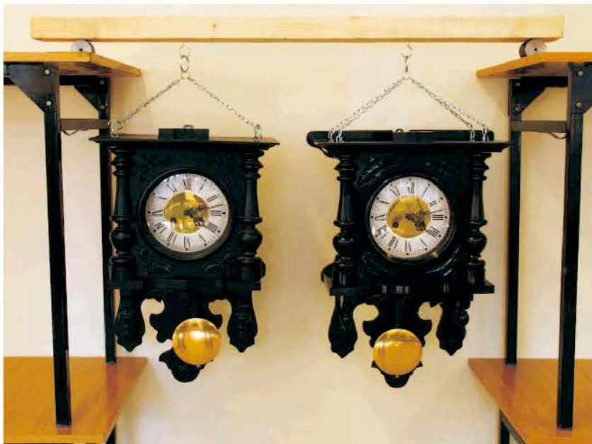
Fig. 2. Experimental setup with two pendulum clocks. (a) Clocks hanging from the wall. (b) Clocks hanging from the shelf. (c) Clocks hanging from the shelf.
